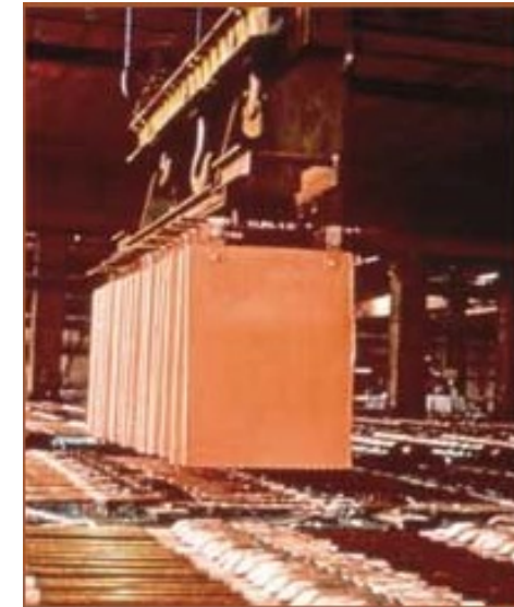
Picture 9. The giant copper cathodes being lifted out of the solution. Notice all the electrolytic cells underneath.
