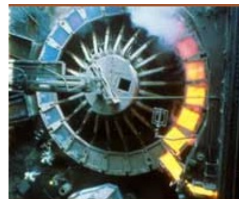
Picture 8. This huge wheel is used to cast the anodes. Molten copper is poured into a mould and the wheel is turned for the next mold. Meanwhile, the molten copper cools and solidifies into anodes over a metre tall.
